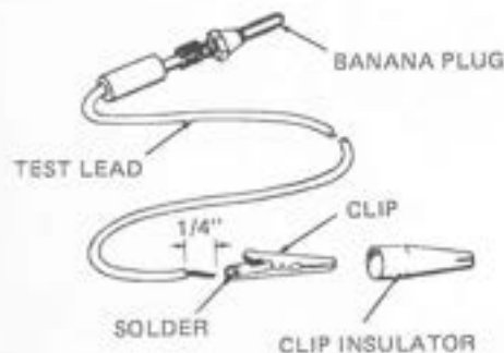
Figure 47. Assembling the test leads.
